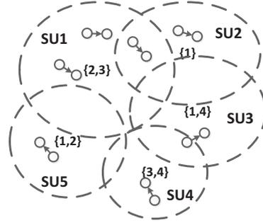
Fig. 2: Collision domain with 5 SUs and each of them has one or more channel demands. The dashed circle denotes the communication range of an SU, and the two small circles connected with an arrow denote the communicating parties.
